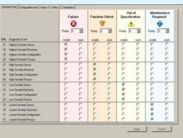
For example, the category MAINTENANCE receives higher importance. It can be marked as highest level by easily checking the related field in the DTM. On the other hand side, a failure of an unimportant event should receive a low ranking. Related checkboxes have to be selected.
