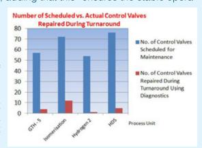
Before using device diagnostics, about 60 percent of the control valves were selected for repair in a typical plant shutdown. While all faulty valves were likely corrected, others may have been removed unnecessarily due to a lack of data. With device data, the company estimates average savings of \$70,000 per unit, per shutdown; it's no longer necessary to disassemble and repair failure-free control valves during a shutdown.
