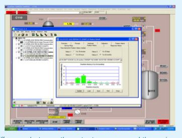
toring of friction (difference between the output pressure and the spring range). An abnormal deviation in this value may highlight a mechanical problem in these valves, prompting preventive maintenance. Pilot functions on digital positioners have allowed Arkema to optimize control loops.
