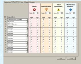
implementation of FOUNDATION fieldbus diagnostics also conforms to NAMUR's recommendations both by distinguishing between device and process problems and by using the standard NAMUR diagnostic FCSM classifications as its standard diagnostic classification.
