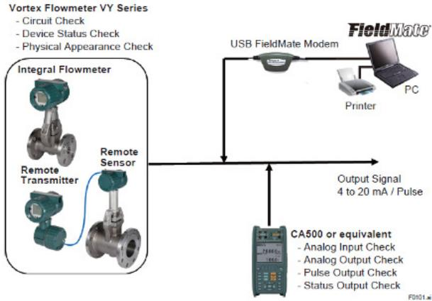
Fig. 6 System configuration
