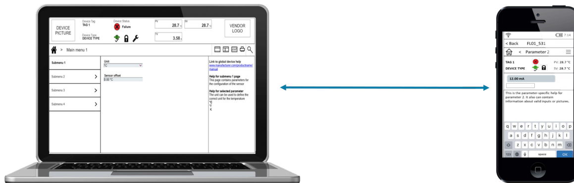
Figure 4. New FDT 3.0 DTMs employ a responsive design approach for use with all types of mobile devices.
